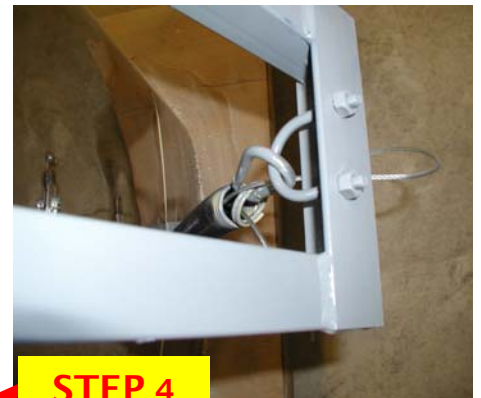
STEP 4 - Raise lid wide open and detach spring, slowly lower lid to closed position
